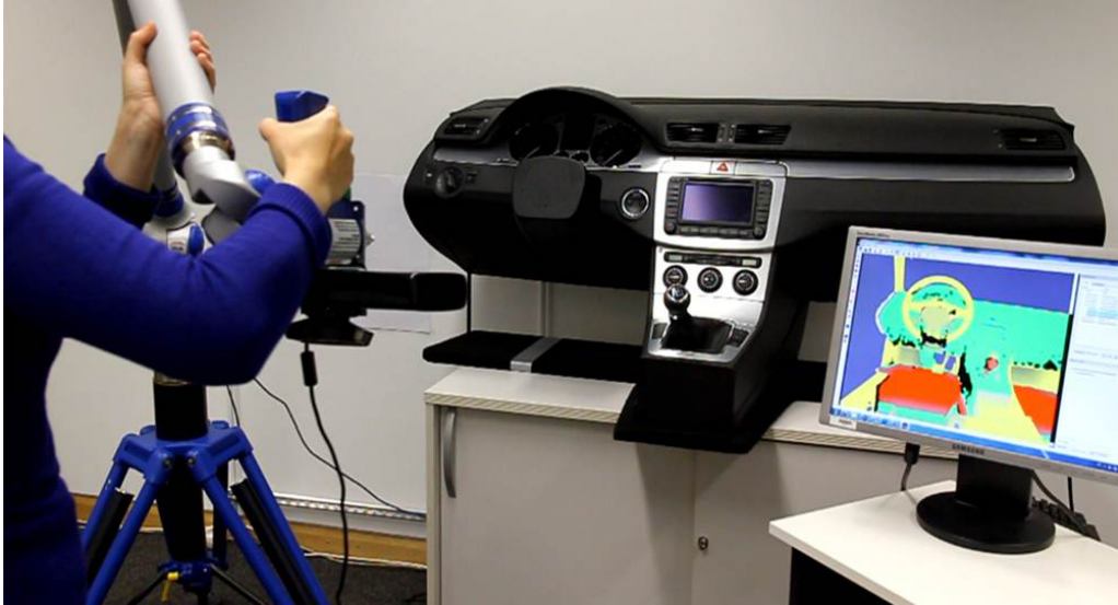
Figure 4: 3D difference detection with a Kinect depth camera and a Faro measurement arm.
