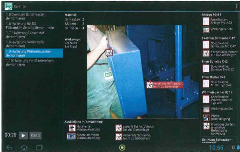
Fig. 6. An exemplary design of an assistance system showing multiple steps of an assembly work task on the left and a detailed description of the current step in the center. Annotations for the work task are embedded directly in the center view as sticky notes (see the two red annotations on top of the image) and summarized below. Additional relevant information regarding related concepts (such as reports to the machine and its parts, specifications of tools and materials) is integrated in a virtual clipboard on the right.
