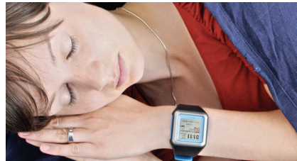
Figure 1: SeismoTracker enables any smart Wearable with an accelerometer to sense vital data, such as: heart rate (HR), respiration rate (RR) and microvibrations (MV) of the muscles. Our approach relies on seismocardiography (SCG), which basically senses low-amplitude movements caused by the users' body functions. This method works flawlessly in resting states, which are for example: a) sleeping b) sitting calmly c) shoring up the body part (e.g. laying down the hand).
