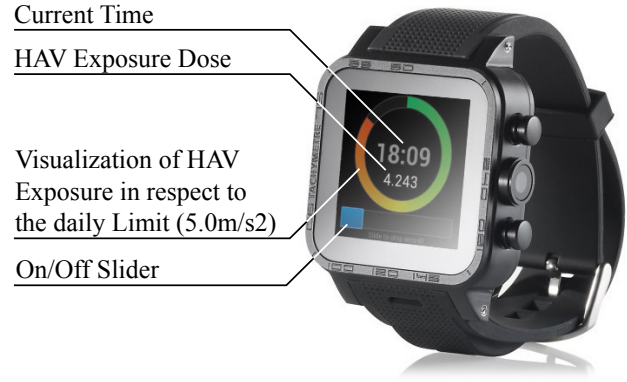
Figure 2. The AGIS Android app running on an autarkic smartwatch (SimValley AW 429 RX).
