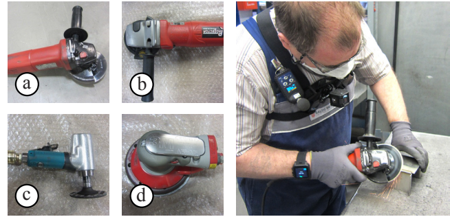
Figure 4. In our pilot study, the worker trained four similar grinders, which were: a) angle grinder Hilti, b) angle grinder Milwaukee, c) pneumatic grinder, d) wobble disc grinder. The AGIS smartwatch system was then distinguishing those and estimating the daily HAV doses.
