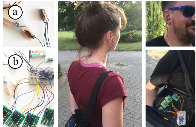
Figure 1. EarFS is a wearable electric field sensing device which enables to sense mobile facial-related gestures. It consists of a) an ear plug plus a reference electrode (a clothes peg that has to be attached to the ear lobe), and b) four sensing shields that are connected to an Arduino which runs on a 9V battery supply and transmits data via Bluetooth.
