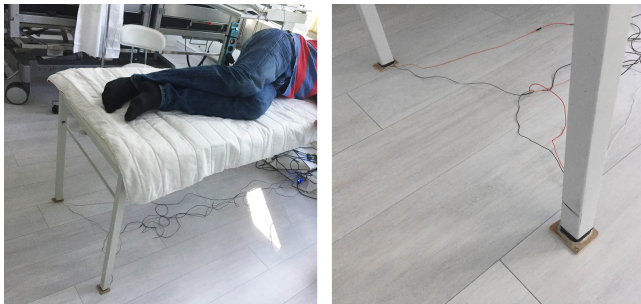
Figure 3: We additionally put Load Cells under the bed poles that additionally measure the pressure exerted on the bed.
